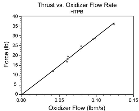
Figure 6. Plot of the thrust vs. oxidizer flow rate for HTPB.
