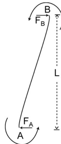
Figure 2. Diagram of a sigmoid beam.
