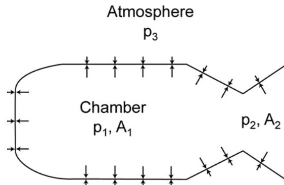
Figure 1. Simplified Schematic of a rocket motor.
