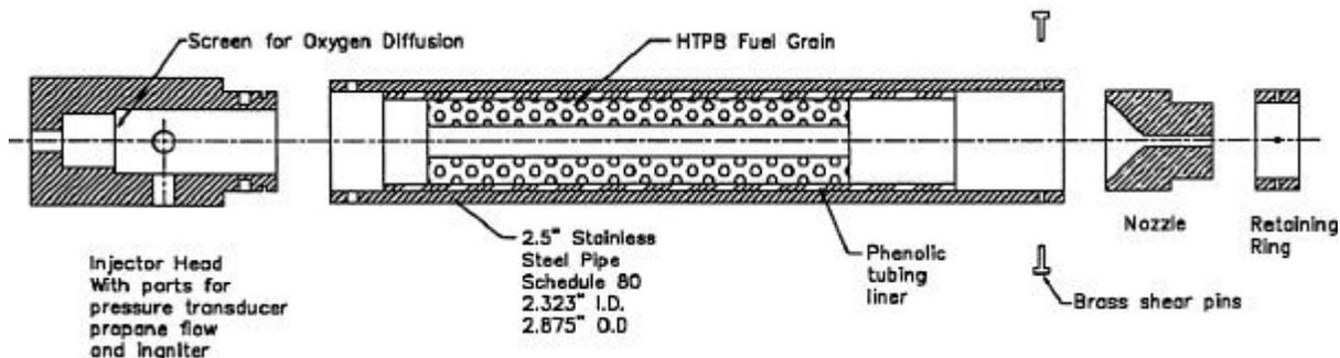
Figure 1. Layout of the lab-scale hybrid rocket motor.
